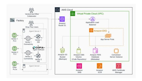
The Amazon EKS cluster is configured to be horizontally scalable. Connectivity between the Factory and the AWS cloud over AWS Direct Connect (or AWS Site-to-Site VPN) keeps all the traffic private and encrypted. This architecture allows Amazon to privately store their code repositories and enable a centralized source management practice for their Automation code. It enables Amazon to standardize code management and code collaboration practice both internally and externally (with vendors).
